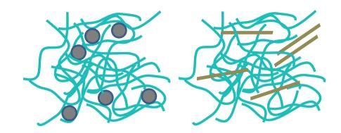
Plastic film can be a mixture of different polymers e.g. polymer blends or layers
