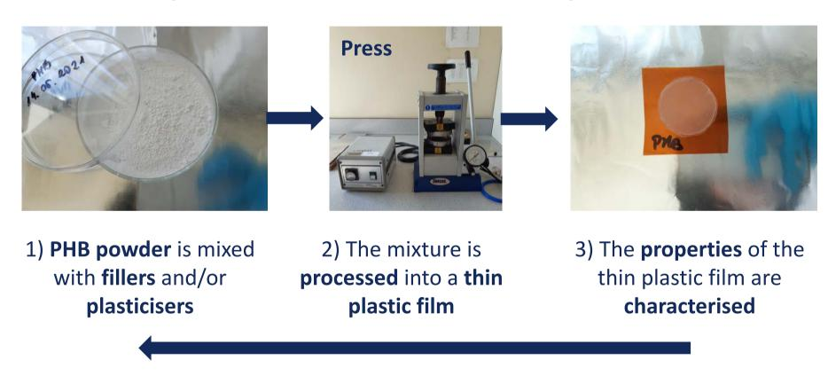
Repeat 1-3 with different components and processing conditions to **optimise the plastic film**.
